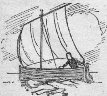
A Dipping Lug—a sail usually set in lifeboats.
